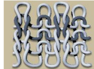
Rib knitted structure
