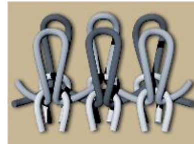
Interlock knitted structure
